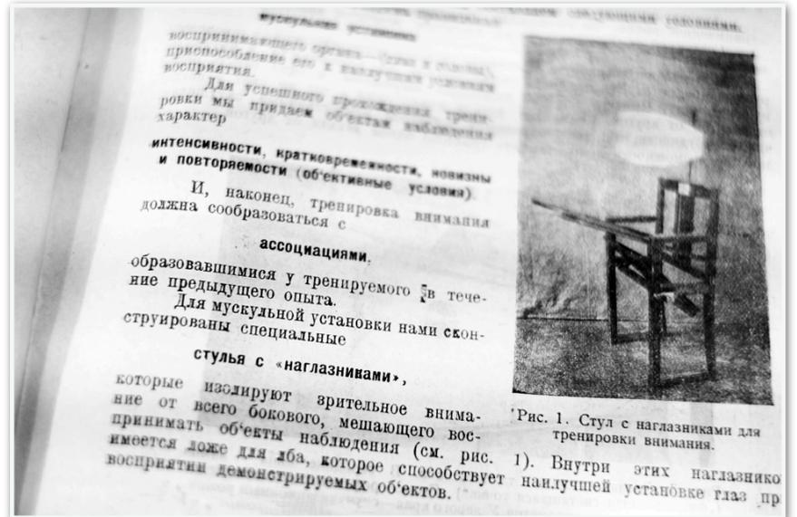
Techniques of the Central Institute of Labour: The curved panel at head height blocks peripheral vision. This was used in exercises to test and improve focus, encouraging workers not to be distracted by other things in their field of vision.
